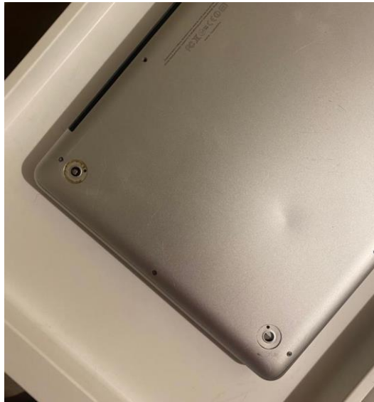
Figure 4.4. The missing screws from the participant's laptop
