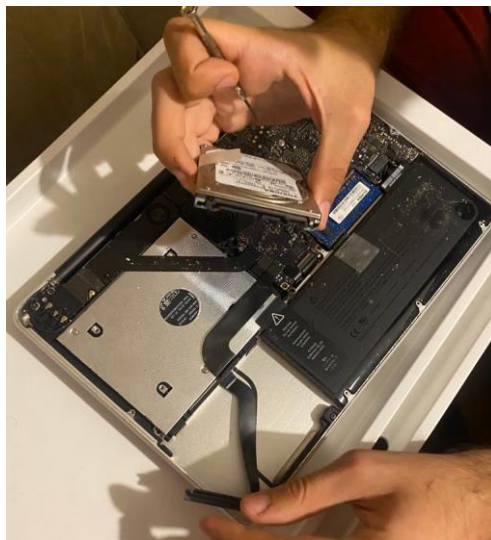
Figure 3.4. Participant 3 replacing the HDD card on his laptop
